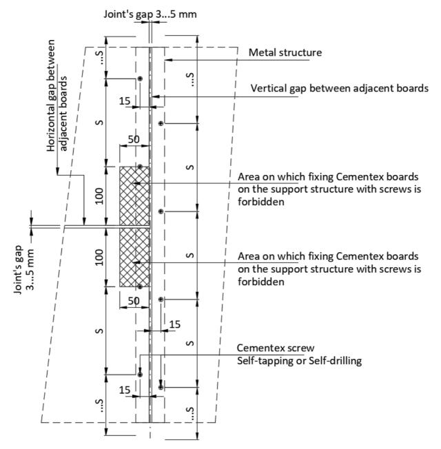
S - Disposal step for the screws used for fixing the Cementex boards on the support structure In the absence of other technical specifications for the project, S = maximum 300 mm
